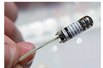
A pinger tag fixed to skipjack tuna
